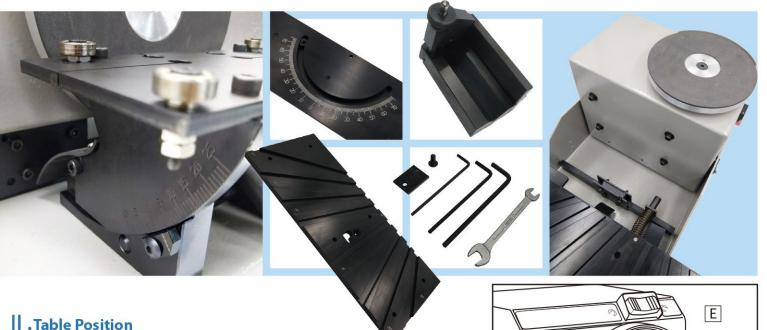
The vertical wheel position allows use of the calibrated table and tool guide. Two tool angles can be simultaneously controlled. Tool clearance (relief) can be adjusted by setting the table elevation. To set table elevation:
